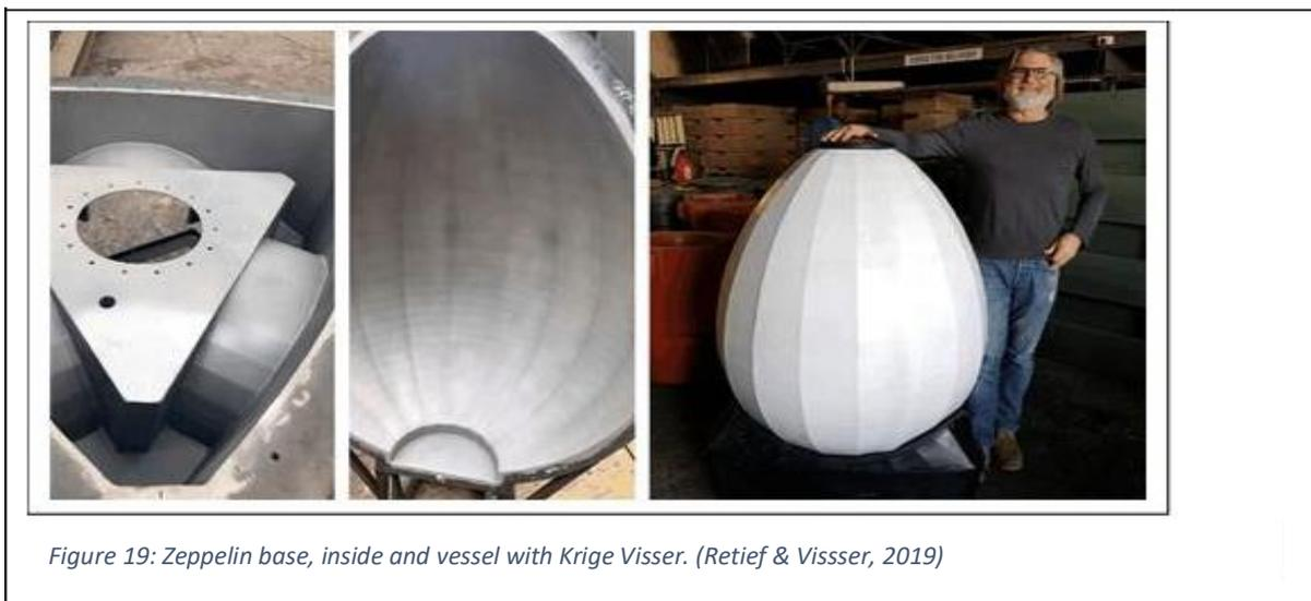
Figure 19: Zepelin base, inside and vessel with Krige Visser. (Retief & Visser, 2019)
