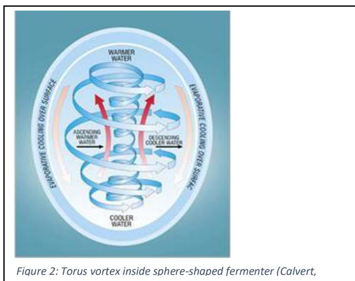
Figure 2: Torus vortex inside sphere-shaped fermenter (Calvert,
