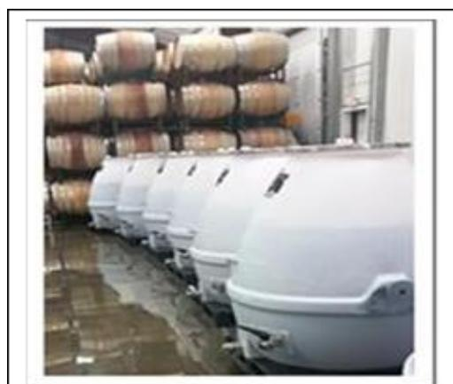
Figure 20: Apollo ovoid vessel, note the flat base, no need for footing structure. (Flextank, 2016)
