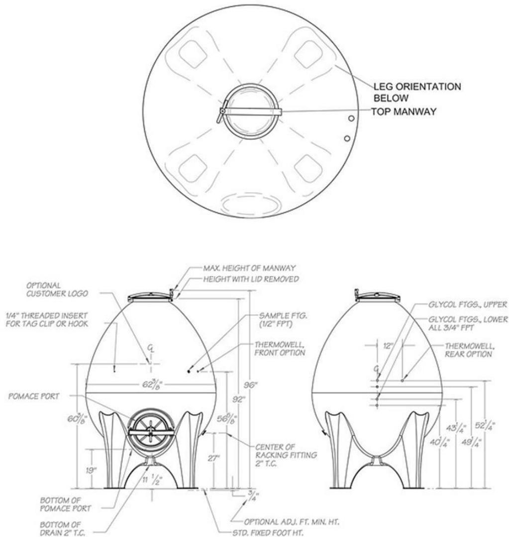
Figure 1: Diagram of cement ovoid wine vessel (Ikapa, 2019)
