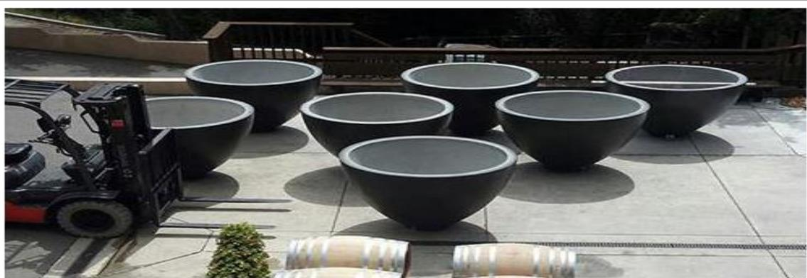
*Figure 10: Teacup wine vessels. ideal for use as open fermenters for small batch winemaking. (SonomaWinetanks, n.d.)*
